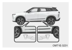
Make sure that the vehicle is on the correct jacking point to avoid damage to high/low voltage cables or power battery when the vehicle is lifted.
