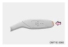
Step 1: Depress brake pedal, and park the vehicle smoothly. When the vehicle is stationary, press P button to switch the gear position to P to activate the parking brake function;
