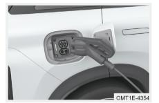
Charging gun has anti-theft function. After inserting charging gun and entering full power charging or when doors are locked, charging gun will be locked automatically.
