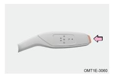
Step 1: Depress brake pedal, and park the vehicle smoothly. When the vehicle is stationary, press P button to switch the gear position to P to activate the parking brake function;
