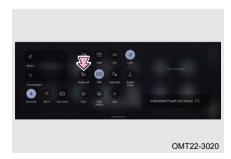
When the vehicle is in a stationary state and the shift position is in P/N, press the power-off switch and confirm to turn off power supply of the vehicle according to the hints on head unit, the vehicle is powered off.
