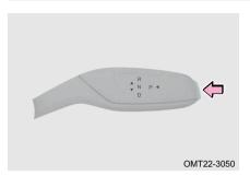
Depress brake pedal, and park the vehicle smoothly. Press P button to shift the gear position to P, "(P)" red indicator on instrument cluster remains on, indicating that parking function is activated.
